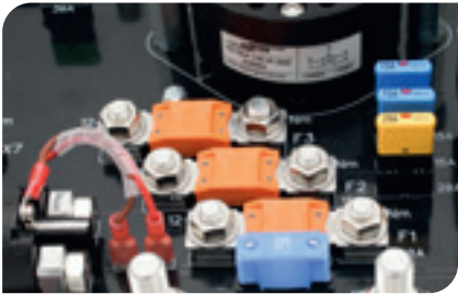
Two power elements with M8 pins at a defined distance for mechanical and electrical connection of mega fuses to the circuit board.
