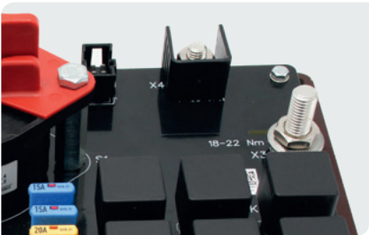
Contact protection around the power element, to prevent the cable lugs connected to the neighbouring power elements touching each other and causing a short circuit.
