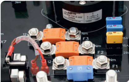
Two power elements with M8 pins at a set distance apart to mechanically and electrically connect a mega fuse to the circuit board.
