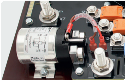
Two angled power elements at a set distance apart to mechanically and electrically connect a high-current relay to the circuit board.
